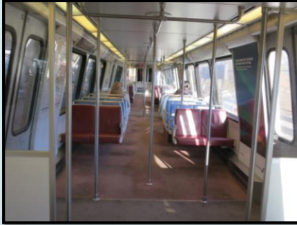
WMATA/D.C. Metrorail Breda 3000 series car delivered in 1987 (pre-ADA) showing floor-to-ceiling stanchions (which are 30 inches apart rather than providing a route 32 inches wide required under the ADA)
