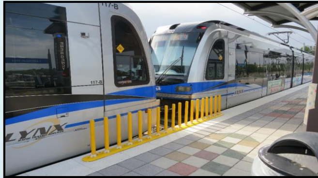
Charlotte Area Transit System (CATS) LYNX Blue Line light rail trains use platform-based Between-Car Barriers
