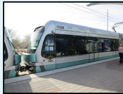
Phoenix Valley Metro Kinkisharyo low floor Light Rail car built in 2008 provides level boarding from platforms about 14 inches Above Top of Rail.
