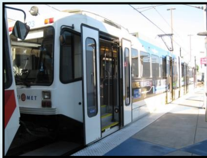
Portland TriMet MAX Bombardier Type I Light Rail car (Built mid-1980s) at platform (note steps inside car). Newer TriMet MAX cars have low floors that are close to platform height.
