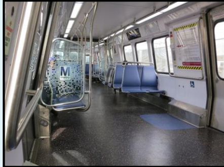
WMATA/D.C. Metrorail Kawasaki 7000 series car delivery began in 2014. Photo shows with open circulation space, wheelchair space that has handholds and handholds attached to seat backs and windscreens and no floor-to-ceiling stanchions
