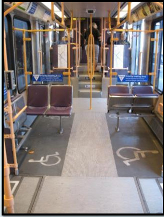
Portland Tri-Met Siemens SD660 light rail car showing two wheelchair spaces and priority seating.
