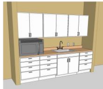
Parallel approach: Allowed in wet bars, and where no cooktop or range is provided (§606.2)
