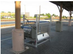
An Amtrak portable platform lift needed to get a wheelchair user or individual unable to climb railcar steps up to a 48 inch Above Top of Rail car floor from a low level platform. The lifts are deployed by the train or station crew.
