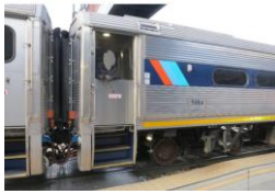
Amtrak California single level rebuilt former New Jersey Transit Comet 1B cars built by St. Louis Car Company for the Penn Central in the late 1960s. The car floor is 48 inches Above Top of Rail. The only means of wheelchair access is by use of a portable platform lift. See upcoming slide.
