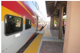
New Mexico Rail Runner Bombardier Bi-Level Commuter car showing raised level boarding platform and bridgeplate in Albuquerque in September 2016
