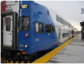
Utah Transit Authority (UTA) Front Runner Bombardier bi-level commuter car at FULL LENGTH LEVEL BOARDING platform in Salt Lake City. Car floors are 25 inches Above Top of Rail. Extended sill at car door appears to mitigate the need for a bridgeplate.
