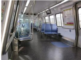
WMATA/D.C. Metro Rail Kawasaki 7000 series car delivery began in 2014. Photo shows with open circulation space, wheelchair space that has handholds and handholds attached to seat backs and windscreens and no floor to ceiling stanchions
