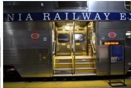
Virginia Railway Express (VRE) Nippon Sharyo Bi-level "Gallery" cars (2006-2008) with center entrance doors with steps up to car floor and equipped with car borne lifts. In photo on right, the left stairway bottom step says "Rincon" which is the maker of the lifts. Gallery cars typically cannot be used at high level platforms. In addition to VRE, similar and older gallery cars are widely used by Metra Chicago suburban lines and Caltrain in San Francisco Peninsula service.
