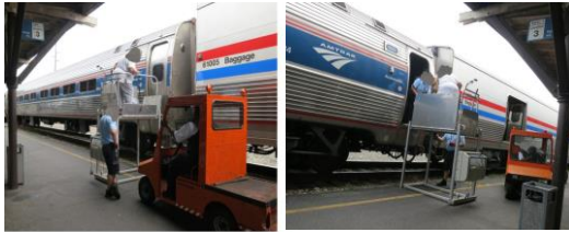
Amtrak personnel have deployed and are assisting an individual to board an Amtrak rail car (with a 48 inch Above Top of Rail car floor) at Raleigh, North Carolina station
