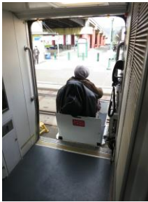
Amtrak California cars have a 18 inch Above Top of Rail car floor. Most passenger platforms in California are no more than 8 inches Above Top Rail and some are at Top of Rail. So a carborne wheelchair lift is needed.
