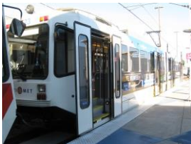
Portland TriMet MAX Bombardier Type I Light Rail car (Built mid 1980s) at low level platform (note steps inside car). Newer TriMet MAX cars have low floors
