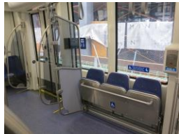
On left, Minneapolis Metro Transit Bombardier Flexity Swift light rail car wheelchair space. Above, Minneapolis Metro Transit Siemens S70 light rail car wheelchair space & priority seating
