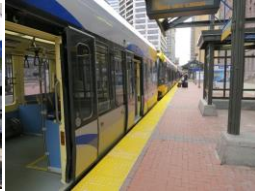
Minneapolis, Minnesota Metro Transit Bombardier Flexity Swift light rail cars with full length level boarding platform
