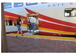
New Mexico Rail Runner Bombardier Bi-Level Commuter car with all passengers boarding from large raised level boarding platform using bridgeplate in Albuquerque in September 2016
