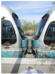
Phoenix Valley Metro, note lack of Between Car Barrier
