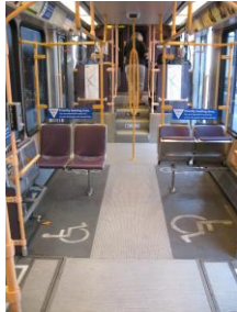
Portland Tri-Met Siemens SD660 light rail car showing two wheelchair spaces and priority seating.
