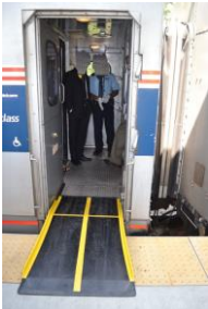
Bridgeplate in use at Amtrak Ann Arbor, Michigan movable set back platform
