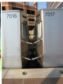
Between-Car Barriers on new Washington DC Metro 7000 series rapid rail (subway) car.
