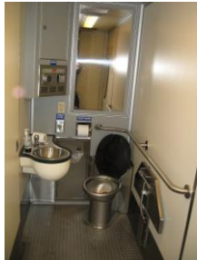
Restroom in Maryland Area Regional Commuter (MARC) Kawasaki MARC III multilevel car
