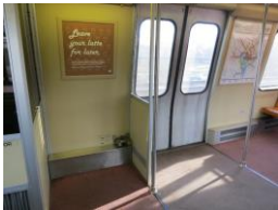
Above, WMATA/D.C. Metro Rail car showing wheelchair space & some floor to ceiling stanchions (poles).
