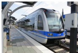
Charlotte Area Transit System (CATS) LYNX Blue Line light rail trains use platform-based Between Car Barriers
