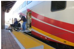
New Mexico Rail Runner Bombardier Bi-Level Commuter car with wheelchair user boarding in Albuquerque from raised level boarding platform using bridgeplate in September 2016. Conductors deploy bridgeplates at every station stop.
