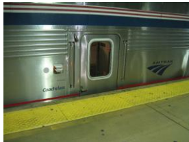
Amtrak Bi-level Superliner car at a 48 inches Above Top of Rail platform at Washington, D.C. Union Station. Floor of car is about 30 inches below the platform
