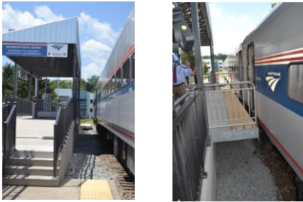
Amtrak's movable set back platform test in Ann Arbor, Michigan. On left, platform is retracted for freight trains clearance. On right, platform extended to provide level boarding onto two cars. Boarding time is shortened and passengers like it.
