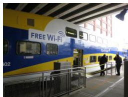
Metro Transit Northstar Target Field Minneapolis station with raised level boarding platform providing access to Bombardier Bi-level commuter car at end of train.
