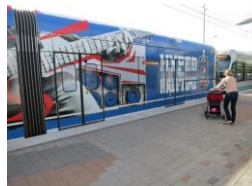
Phoenix Valley Metro Kinkisharyo low floor Light Rail car built in 2008 provides level boarding from platforms about 14 inches Above Top of Rail.
