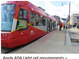
Apply ADA Light rail requirements – Photo shows a Washington, D.C. Streetcar Inekon Trio. Modern streetcars are low floor and often have slightly raised platforms that provide level boarding.
