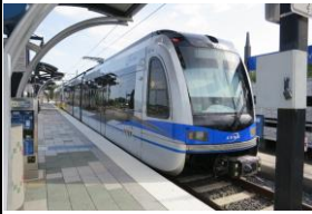
Charlotte Area Transit System (CATS) LYNX Blue Line Siemens S70 light rail cars with full length level boarding platform
