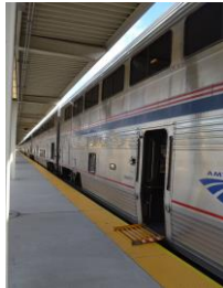
Amtrak's Lorton, VA station provides full length level boarding onto Superliner cars but a bridgeplate is still needed to span the horizontal gap.
