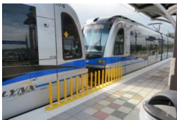
Charlotte Area Transit System (CATS) LYNX Blue Line light rail trains use platform-based Between Car Barriers
