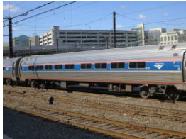
Amtrak Amfleet I single level cars, coach class, built 1975-78. (Pre-ADA). Car floor height is 48 inches Above Top of Rail.
