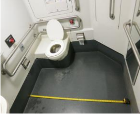
Above, accessible restroom on lower level of Amtrak California bi-level car (which is sort of a hybrid between a commuter rail car and an intercity rail car). The maximum dimensions of the restroom are approximately 65 inches by 75 inches.
