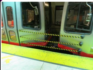
Between-Car Barriers on San Francisco Muni Light Rail cars at a high level boarding subway station platform, installed in 2014.
