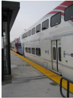
Utah Transit Authority (UTA) Front Runner Bombardier bi-level commuter car at FULL LENGTH LEVEL BOARDING platform in Salt Lake City. Car floors are 25 inches Above Top of Rail. Extended sill at car door appears to mitigate the need for a bridgeplate.
