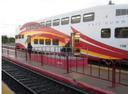
New Mexico Rail Runner Bombardier Bi-Level Commuter car with wheelchair user boarding in Albuquerque from wooden mini-high platform using bridgeplate in October 2011
