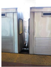
Maryland MTA Metro rapid rail/ subway cars non-cab ends do not have any between car barrier.
