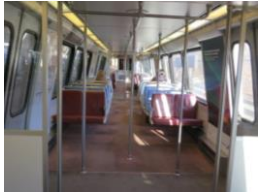
WMATA/D.C. Metro Rail Breda 3000 series car delivered in 1987 (pre-ADA) showing floor to ceiling stanchions (poles) (which are 30 inches apart rather than providing a route 32 inches wide required under the ADA)
