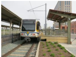
Sacramento Regional Transit light rail car stopped by boarding platform to allow boarding by wheelchairs users and others unable to climb steps onto high floor light rail cars.
