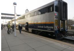
Amtrak California Bi-level California cars (this car built by Morrison-Knudsen in the mid-1990s) have a 15 inch Above Top of Rail lower car floor. Because station platforms are lower, they have carborne lifts on most cars.
