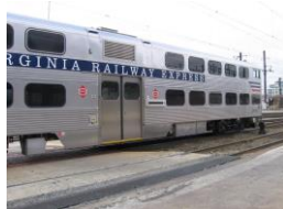
Virginia Railway Express (VRE) Nippon Sharyo Bi-level "Gallery" cars (2006-2008) with center entrance doors with steps up to car floor and equipped with car borne lifts. In photo on right, the left stairway bottom step says "Rincon" which is the maker of the lifts. Gallery cars typically cannot be used at high level platforms. In addition to VRE, similar and older gallery cars are widely used by Metra Chicago suburban lines and Caltrain in San Francisco Peninsula service.
