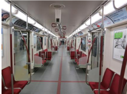
Bombardier TORONTO Rocket, TORONTO, CANADA (not covered by the ADA) but a similar design with full width gangways is specified for next NYC subway order 44
