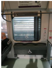
Phoenix Valley Metro Kinkisharyo light rail car wheelchair space and priority seats and signage
