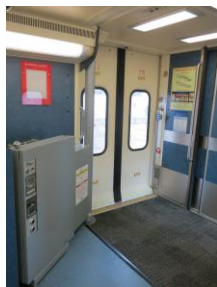
Above, Minnesota Northstar station, raised level boarding platform with bridgeplate deployed. On Right, interior view of car doors with car borne lift (in every car)
