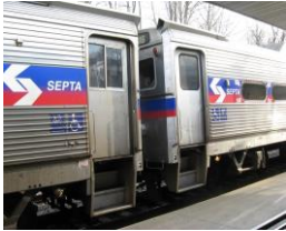
SEPTA GE Silverliner IV (Built 1973-1976) single level commuter car. Car floor is 48 inches Above Top of Rail (ATR). Newly constructed low platforms must be 8 inches Above Top of Rail. Existing platforms are often much lower.
