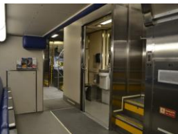
Virginia Railway Express Nippon Sharyo Bi-level "Gallery" cars showing door open to restroom, stairs to galley seats, wheelchair space and priority seating and entrance stairs
