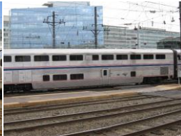
Amtrak Superliner Bi-Level cars. Car #32038 is a sleeping car built in 1981. (Pre-ADA) Car floor height is 18 inches Above Top of Rail.
